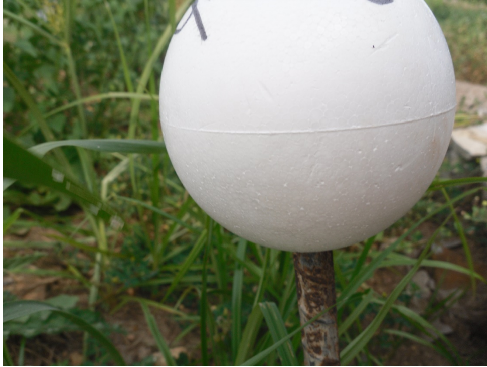
Figure 2.7 Up-Close Image of an Example Control Point.
